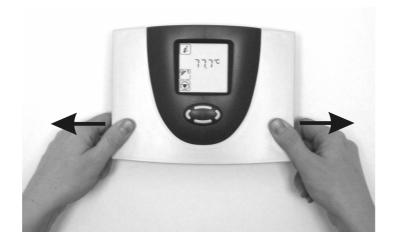
Holding the casing at each side, pull firmly towards you and then raise the top part of the casing until it engages. You can now install and wire up the control unit.
